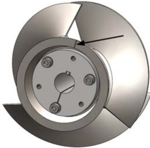
Figure 31. Position of the wedge groove
